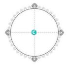
Attach the springs to the jump mat Attach the more tightly curled end of the springs to the D-rings on the jump mat.
