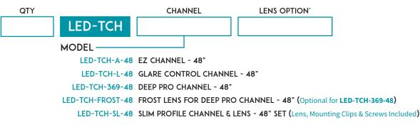
\*Lens Option - Specify <u>LED-TCH-FROST-48</u> if needed for <u>LED-TCH-369-48</u> Channel <u>LED-TCH-SL-48</u> - Sold in a set of Channel & Lens
