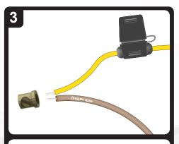
Connect homerun wire with writing to one side of fuse link (except for FHUB).
