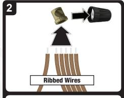
Connect all ribbed fixture wires to the ribbed homerun wire. Insert all wire joins into provided grease cap.
