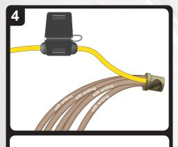
Connect fixture wires with writing to other side of fuse link.
