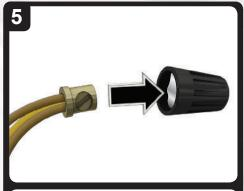
Insert all wire joins into provided grease cap. Thread on cap.
