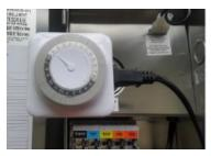
Insert the timer into the outlet on the transformer as shown.
