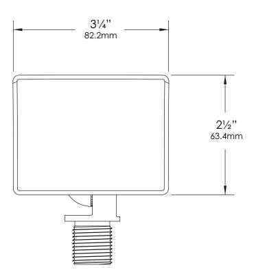
Die-cast brass adjustable knuckle with  $\frac{1}{2}$ " NPS thread. Fixture may be
